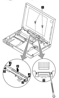
The status indicator has three latches on its rear side and one on its front side. For step **3**, do the following:
